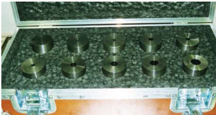
Figure 3 Tungsten collimator and attachment of Linac system for pencil beam
