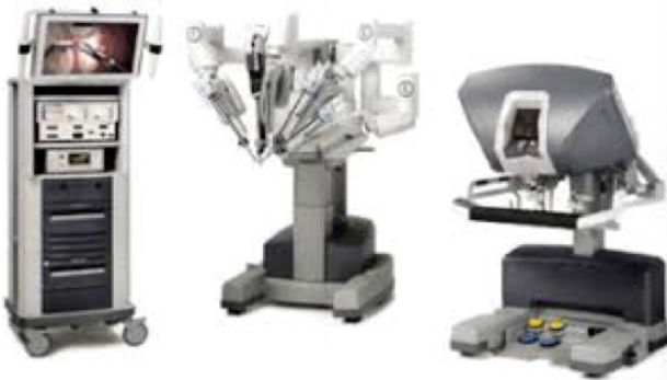
Figure 3 Intuitive Da Vinci surgical system
